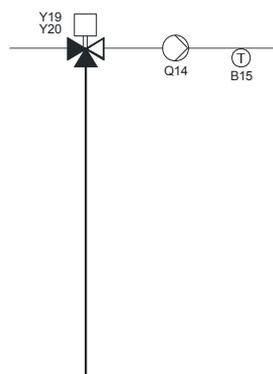
The primary controller allows lower or higher flow temperatures by mixing to obtain flow temperatures for heating/cooling zones with setpoints higher or lower than those of the common flow.
