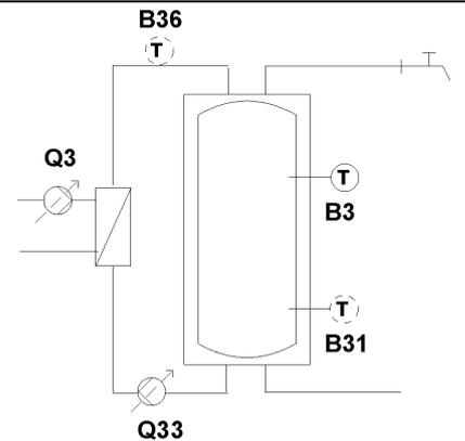
*Heat exchanger outside the storage tank, with primary controller.*
