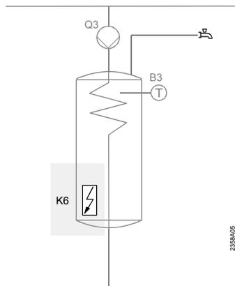
If DHW charging is interrupted because the heat pump exceeded the permissible number of charging attempts (line 2893), the electric immersion heater (K6) – if installed – completes the charging process.
