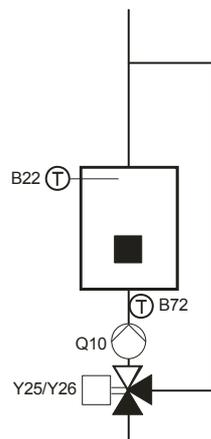
When the temperature of the solid fuel boiler is high enough, the boiler pump is activated and the DHW storage tank and/or the buffer storage tank are charged.
