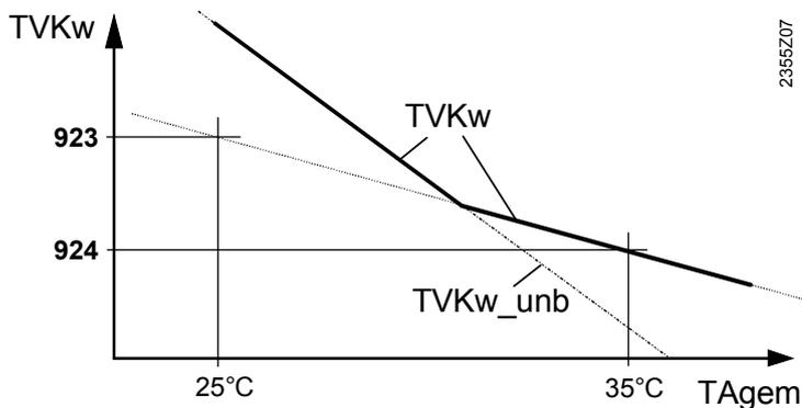
TVKw Flow temperature setpoint for cooling (with minimum limitation)
