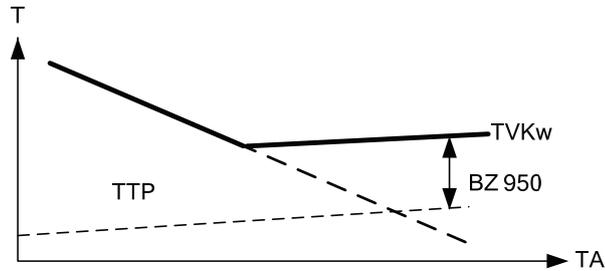
TVKw Flow temperature setpoint cooling
