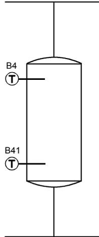
A buffer storage tank can be integrated in the plant. It can be charged via the heat pump, by solar energy or by an electric immersion heater.
