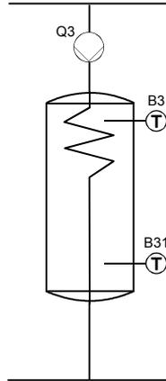
The unit controls the DHW temperature according to the time program, or continuously, to the required setpoint. Priority of DHW charging over space heating can be selected.
