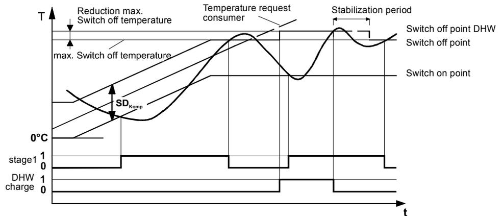
Behavior of Q9 with buffer storage tank at the maximum switch-off temperature
