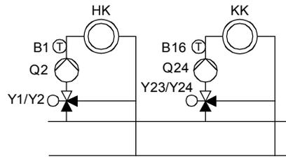
Cooling and heating circuit draw their cooling energy/heat from the same common flow.
