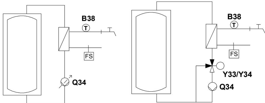
When the DHW flow switch (FS) detects flow, sensor B38 provides control to the nominal setpoint (line 1610).
