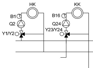
The cooling and heating circuits draw their cooling energy/heat from separate common flows.
