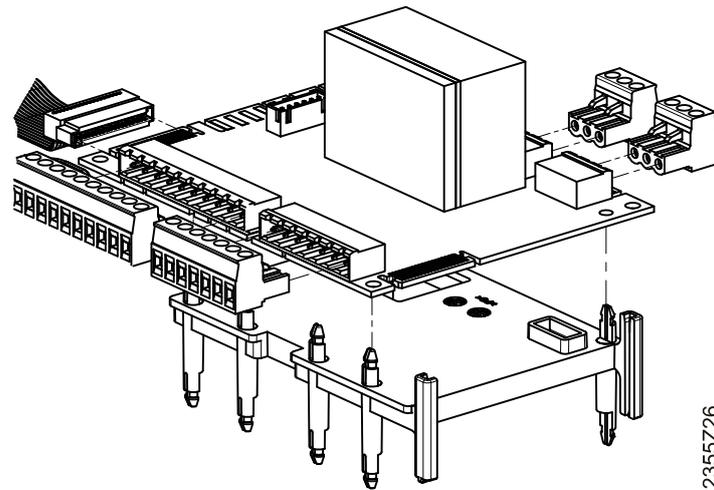
Then, plug the spacer plate together with the I/O module onto the basic unit.
