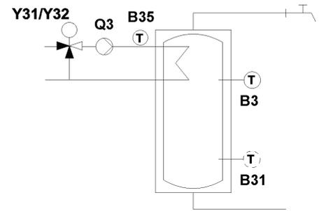
**Speed control charging pump Q3/intermediate circuit pump Q33**
