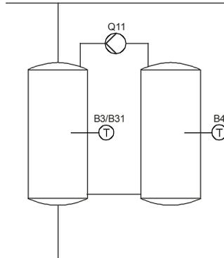
If the temperature level of the buffer storage tank is high enough, the DHW storage tank can be charged by the buffer storage tank.
