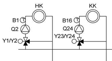
The cooling and heating circuits draw their cooling energy/heat from the same common flow.
