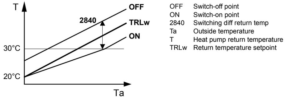
**i** Calculation of the return temperature setpoint is explained on operating line 5810 ("Differential HC at OT -10°C").
