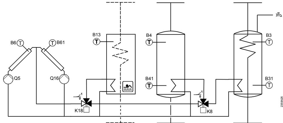
If sufficient solar energy is available, the solar plant can heat the swimming pool, the DHW storage tank and the buffer storage tank. Priorities for heating or charging the different storage tanks can be selected. The pumps can be speed-controlled. Protection of the plant is ensured by a "Frost protection" and an "Overtemperature protection" function.
