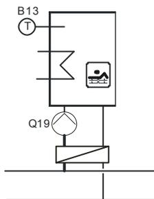
The controller facilitates swimming pool heating with solar energy or via a heat pump using separately adjustable setpoints. In the case of solar heating, it is possible to select priority of swimming pool heating over storage tank charging.
